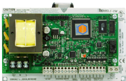
b3887-L-230 Terminal Controller
