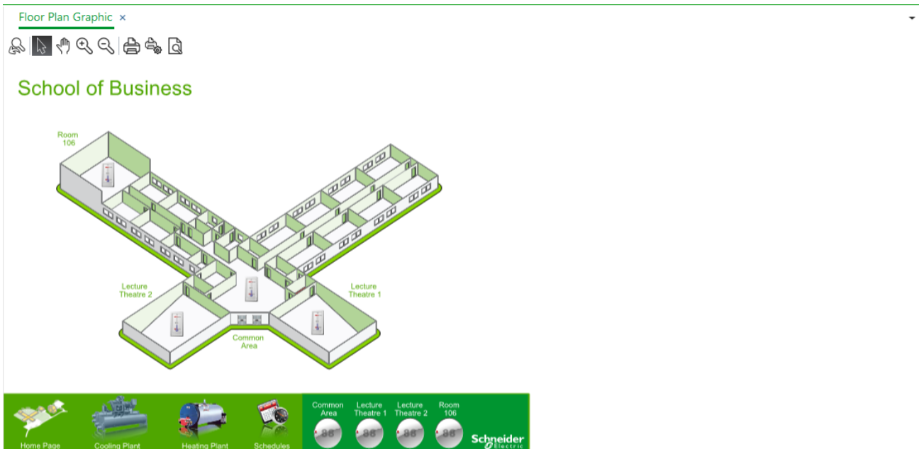
Figure – A Graphic with links and interactive components like gauges in WorkStation
