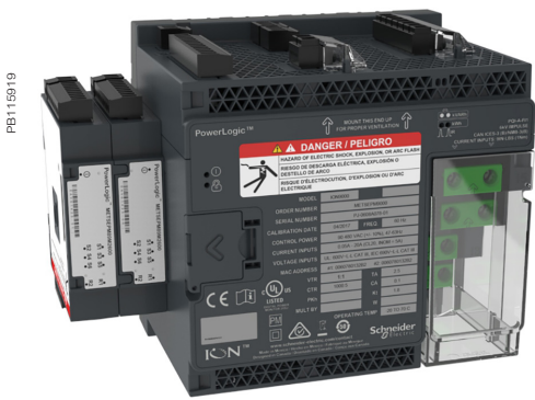
PowerLogic™ ION9000 front with two option modules
