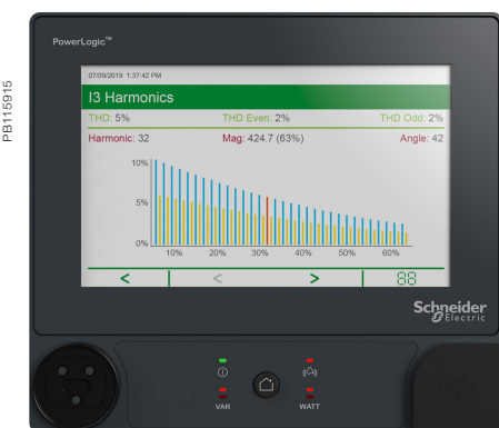
PowerLogic™ ION9000 Harmonics display
